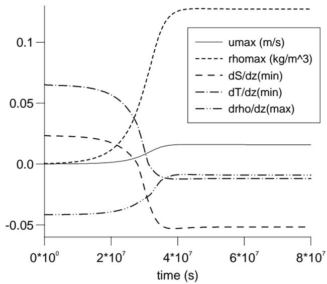
Figure 2: Maximum zonal velocity and density perturbation along with the minimum values of vertical gradients of temperature and salinity and the maximum value of the vertical density gradient.  $10^7\text{s} \approx 100$  days. Units are  $\text{psu/m}$  for  $\partial S/\partial z$ ,  $\text{K/m}$  for  $\partial T/\partial z$  and  $\text{kg/m}^4$  for  $\partial \rho/\partial z$ .
