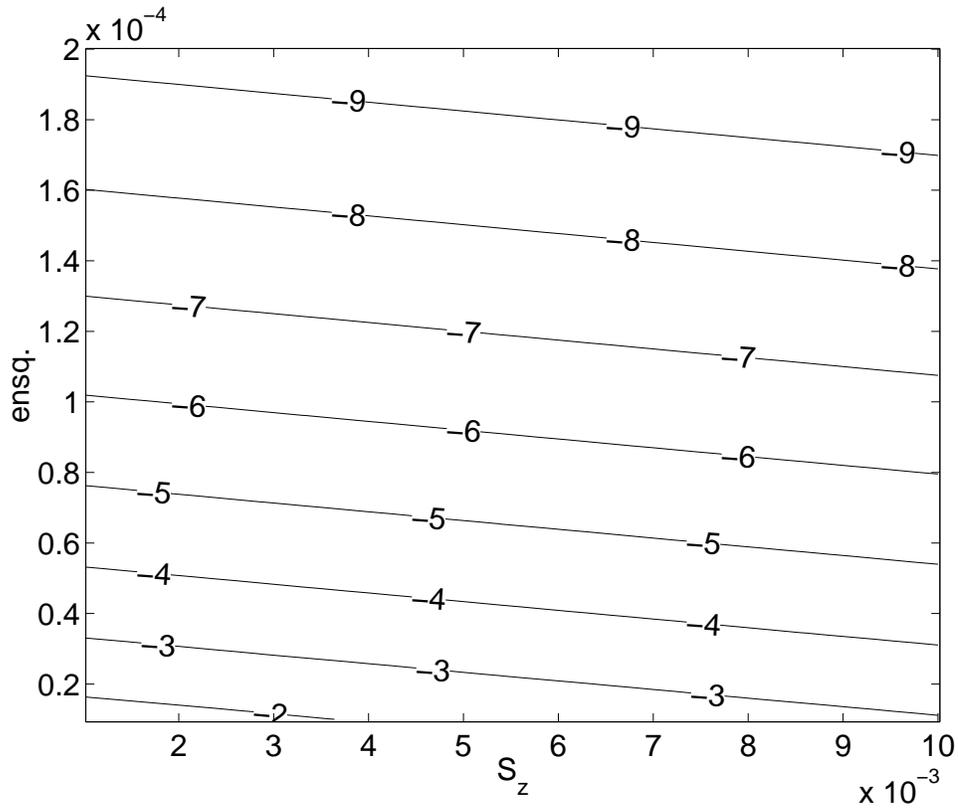
Figure 7: The value of  $\bar{S}_y$ , in  $10^{-6}$  psu  $m^{-1}$  at which the linear growth rate equals  $10^{-7}$   $s^{-1}$  as a function of  $N^2$ , in  $s^{-1}$ , and  $\bar{S}_z$ , in psu  $m^{-1}$ .
