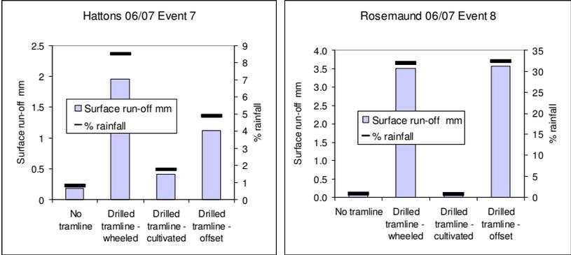
Figure 3. Total over-winter surface runoff at Hattons 2006/07 showing replicate data
