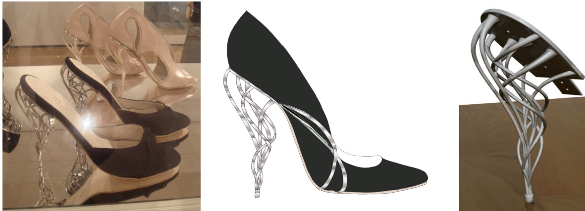
Figure 2 Rapid prototyping model of the heel, final shoe and sketch above
