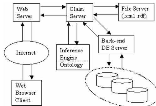
**Fig. 2.** Architecture of the ClaiMaker Claim Server
