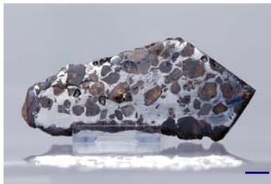
Figure 1. Metal rich example of Main Group pallasite Brahin, scale bar 1cm
