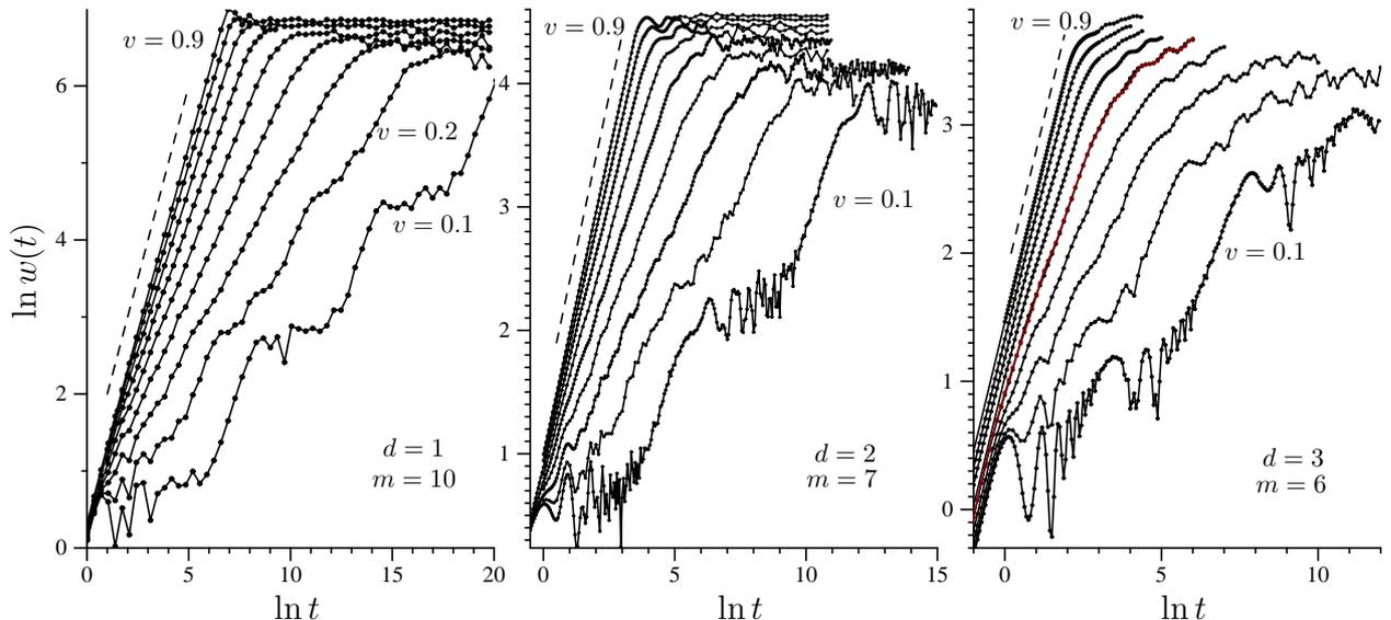
FIG. 6: Calculated values of the width  $w(t)$  of the wave packet for three systems as indicated in each panel, for  $v = 0.9, 0.8, \dots, 0.1$ , going from top curve to the bottom, respectively. The dashed line in each panel has slope 1 corresponding to the ballistic motion.
