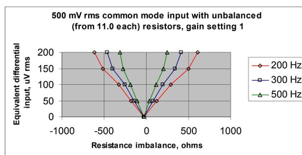
The effect of isolation was investigated next. Common mode signals may be injected via the large capacitance between the input and output commons. If there is an interference source between the body and the 0V lead, a proportion of the interfering signal appears on the centre contact via the potential divider formed by the capacitance and the contact impedance, as shown below.
