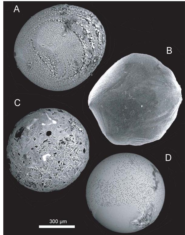
**Figure 1:** Back-scattered electron images. **A-B,** Barred olivine cosmic spherules for which oxygen isotope ratios show relationship with carbonaceous chondrites (A) and ordinary chondrites (B). **C,** Porphyritic olivine cosmic spherule. **D,** Glassy cosmic spherule.
