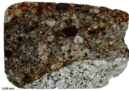
Figure 1. Plane light image of the thin section, shows distinct lithologies of the L3-6 host and the coarse-grained clast (lower right). Note the 5.00 mm scale bar.
