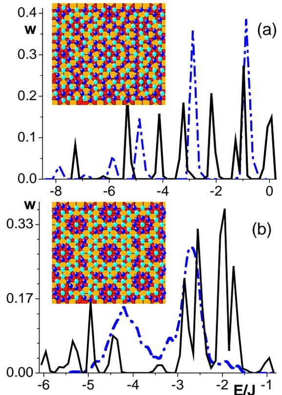
FIG. 2: The frequency distribution of the energy per spin on the octagonal tiling for (a) Ising and (b) vector spins. Solid lines correspond to the case  $J_d < 2J$ , dashed lines to  $J_d > 2J$ . Purely antiferromagnetic interaction at  $kT = 0.01J$  is considered. Top-views of portions of Monte-Carlo configurations with underlying tilings are shown as insets. The light and dark circles represent different spins in (a) and different energies in (b), respectively.
