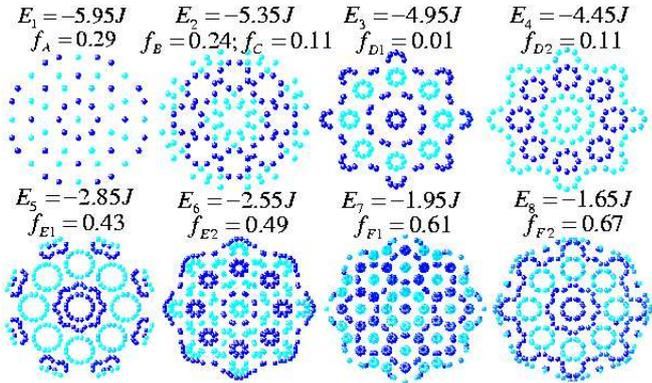
FIG. 3: (color on-line) Spatial distribution of magnetic moments belonging to eight sub-tilings of a noncollinear configuration on an octagonal tiling consisting of 2193 spins.  $J_d > 2J$ . The light and dark circles represent positive and negative  $x$ -components of the magnetization. The in-plane components are not given for the sake of simplicity. Average values of the exchange energy  $E$  and the local frustration  $f$  per spin are indicated.
