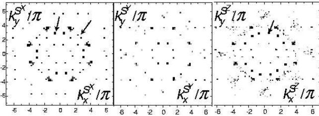
FIG. 5: The calculated Bragg scattering of  $S^x$ ,  $S^y$  and  $S^z$  component of magnetization for the antiferromagnetic superstructure. Reflexes indicated by arrows are new in comparison to previous studies [5].
