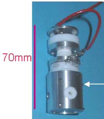
ial through the wall of the penetrator, either in direct line-of-sight, or through a deployable fibre-optic cable. Figure 5 shows a prototype, ruggedised ion trap mass spectrometer developed by the Open University.
