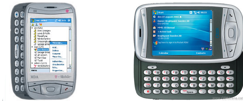
Figure 1 (left): Windows menus on a smartphone similar to the one in this study. Right (Qtek 9100): the screen reformats into landscape when keyboard is pulled out. (Left: http://qtek-smartphone.handster.com/software.php?id=90&for=Qtek+Smartphone; accessed 10 April 2008. Right: http://www.gsmarena.com/qtek_9100-pictures-1257.php; accessed 14 April 2008)
