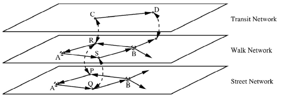
**Figure 8: Conceptual diagram of the Planner Network. Parking accessories are in the Street Network, activity locations in the Walk Network, and transit stops in the Transit Networks from Barrett et al. (1999).**
