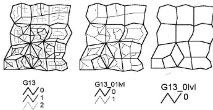
**Figure 3: A graph with three hierarchical levels: (left) full graph containing all nodes and edges (lowest level); (middle) a subgraph containing only two levels of detail; (right) the smallest subgraph containing only the highest level (0-level) from Car et al. (2001).**
