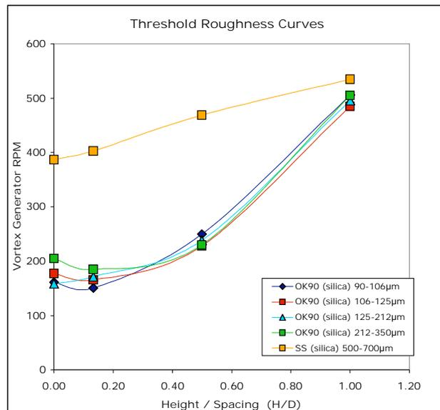
**Figure 2.** A plot of roughness curves for silica sands tested in this study. The height/spacing ratio ( $H/D$ ) is a measure of the surface roughness where increasing values correspond to increasing roughness. Vortex generator RPM is roughly analogous to tangential velocity of the vortex.
