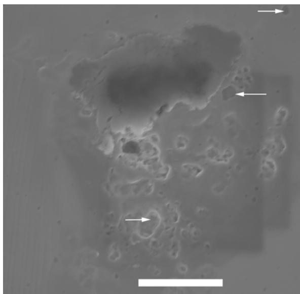
Fig. 1a. Backscattered electron (TLD) image of C2005,2,121,1,0. White arrows point to some of the iron oxide grains. The main mass is mainly composed of aerogel. The substrate is Au. Scale bar 5  $\mu\text{m}$ .
