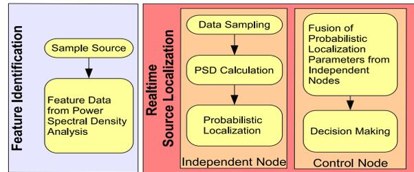
**Figure 1. Block Diagram of Proposed Source Localization using Power Spectral Analysis and Decision Fusion**
