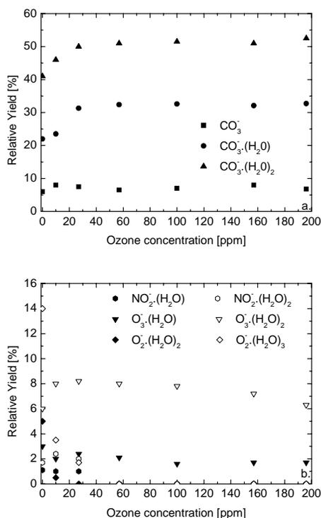
Fig. 4 a., b. The dependence of relative yield of major (a.) and minor ionic species in spectra on ozone concentration in flowing ozonised wet air.
