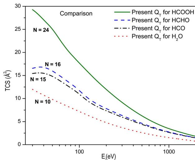
FIG. 5. (Color online) Comparison of the TCSs for different targets ( $N$ , number of target electrons). Solid line, present  $Q_T$  for HCOOH. Dashed line, present  $Q_T$  for HCHO. Dashdot line, present  $Q_T$  for HCO. Dotted line, present  $Q_T$  for H $_2$ O.
