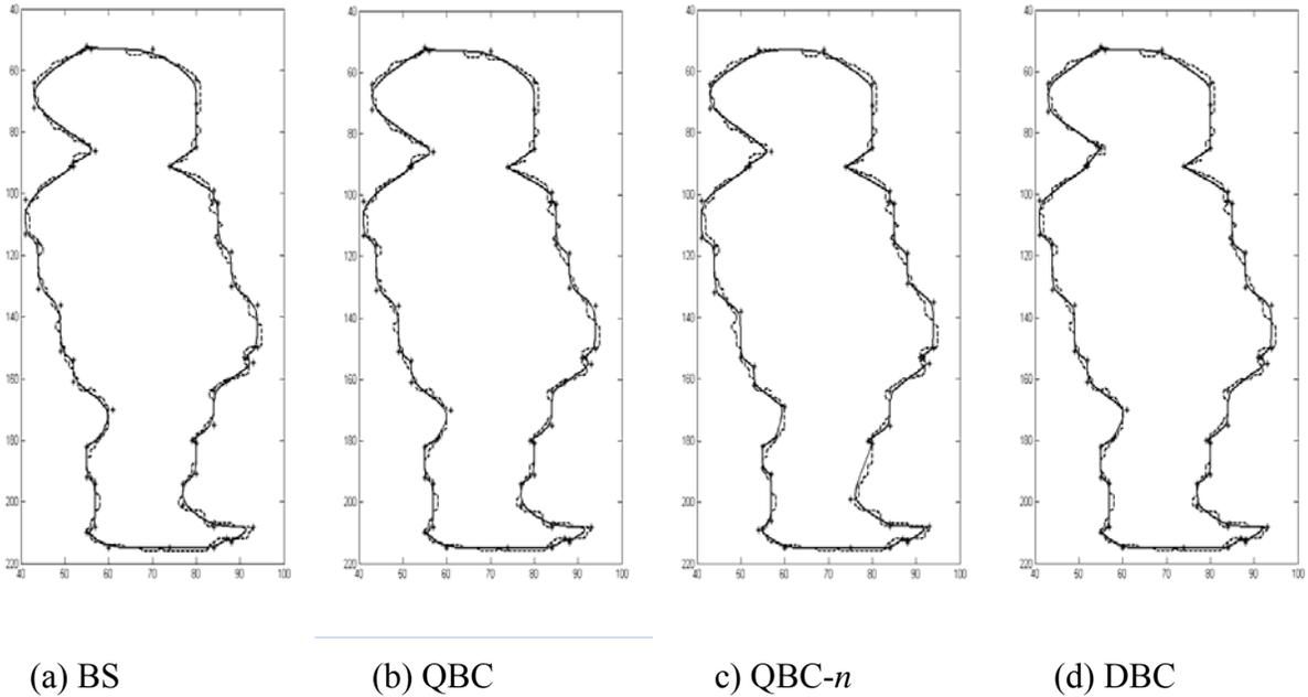
Figure 14: Results for the left-hand kid in the 1<sup>st</sup> frame of the *Kids* sequence with  $T_{\max} = 2$  and  $T_{\min} = 1\text{pixel}$  (legends – *solid line*: Approximated boundary; *dashed line*: Original boundary; *asterisk*: CP).
